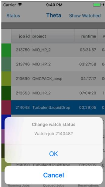
**Figure 4:** The Jobs Table displays all running jobs, queued jobs and reservations for a machine. Users can select jobs to track, or “watch.”
