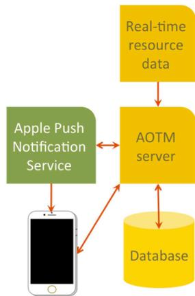
**Figure 1:** The AOTM server tracks each device that has registered for push notifications and that device’s app settings. It organizes the real-time resource data in its database and determines when push notifications need to be sent to a device. When it has determined that a notification needs to be sent, the AOTM server asks the Apple Push Notification Service (APNS) to execute the push notification. The APNS also lets the AOTM server know when a device has been unregistered.
