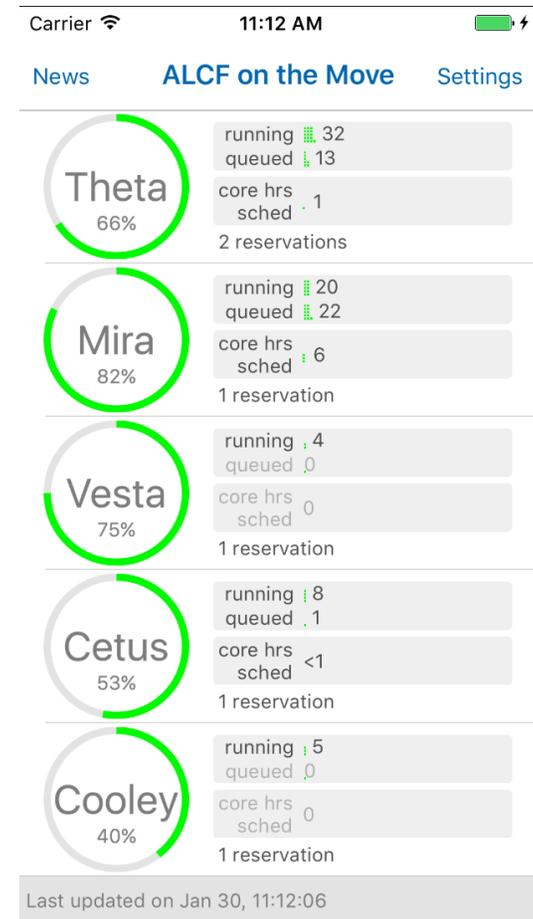
**Figure 2:** The ALCF Dashboard gives users a glanceable overview of the state of ALCF supercomputing resources, in real time.
