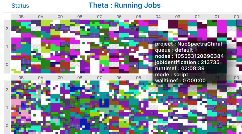
**Figure 3:** Snapshot of the Map screen showing jobs running on Theta. The Map tool [OK?] helps users see the current utilization of a specific resource. Job information can be displayed by selecting any nodes running that job.
